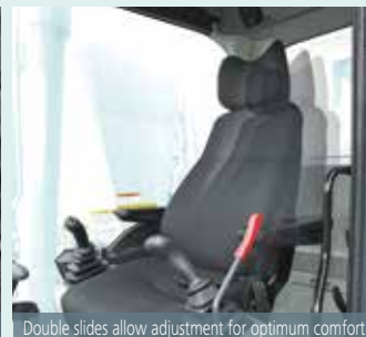
Double slides allow adjustment for optimum comfort
